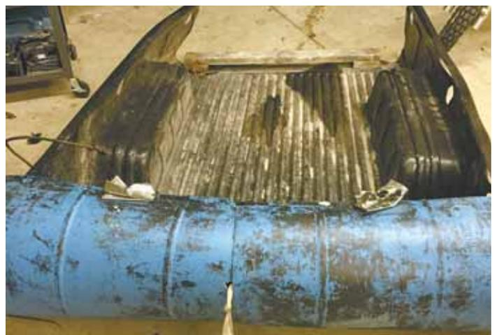
Setcoski cut a 55-gal. plastic barrel in half lengthwise to make 2 halves, then bolted them on front of plastic pickup bed liner.
