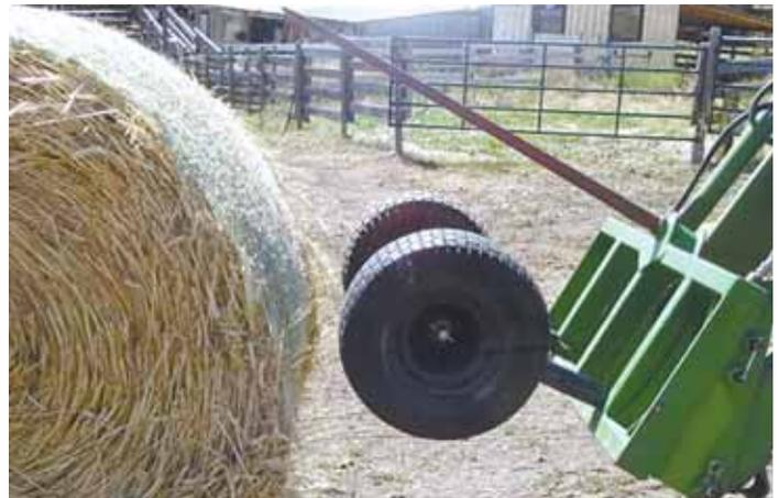
Two-wheeled unroller fits onto a pair of 2-ft. long stabilizer bars on loader-mounted bale spear.
