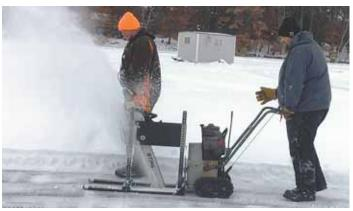
To cut the ice they use a chainsaw secured on a "Chainsaw Chariot" built out of a tracked snowblower.
