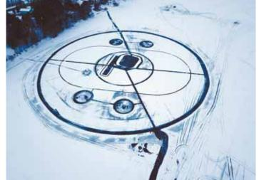
Giant powered ice carousel measures 508 ft. in dia. and is rotated by 4 electric trolling motors. Four smaller carousels were cut into the big one.
