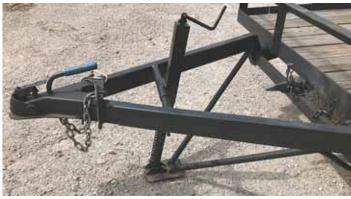
TripleQuick Jack comes with a quick-drop leg so you don't have to crank it down every Jack automatically rotates back and lifts itself out of the way as it's cranked back up. time you use it.
