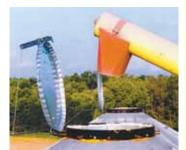
Bin cap opens and closes by pulling on or releasing a cable that runs down to ground level.
