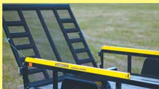
Tailgate lift assist consists of two 6-ft. lengths of square tubing that bolt onto trailer side rails. You can easily lower tailgate with your finger and lift it with your toe.
