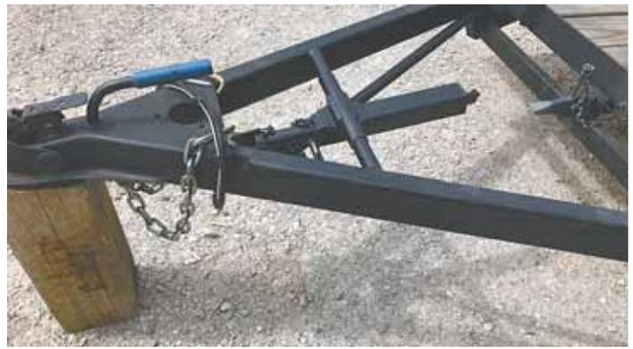
Jack automatically rotates back and lifts itself out of the way as it's cranked back up.
