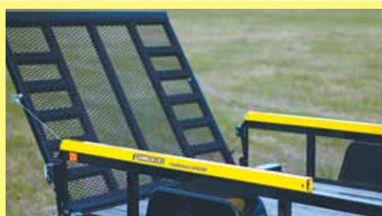
Tailgate lift assist consists of two 6-ft. lengths of square tubing that bolt onto trailer side rails. You can easily lower tailgate with your finger and lift it with your toe.
