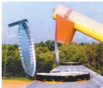
Bin cap opens and closes by pulling on or releasing a cable that runs down to ground level.
