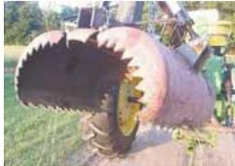
A pair of hydraulic cylinders open and close air tank jaws, which have "zig zag" teeth that grab loads firmly.
