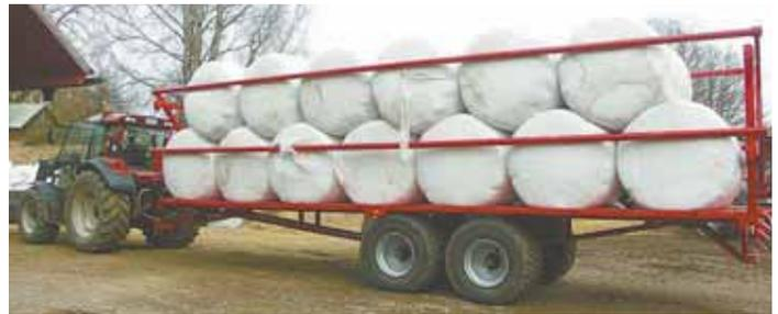
Trailer's retractable side rails eliminate the need for straps when hauling big bales. This 40-ft. model can carry up to 30, 4-ft. dia. round bales or up to 60 big squares.
