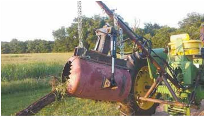
Will Bass started with an old 3-ft. long, 20-in. dia. air tank to build his boom-mounted "clamshell" grapple.
