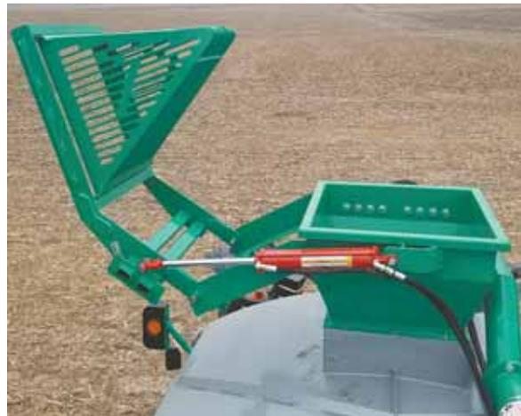
Trash Basket attaches to fill port on liquid manure spreaders and filters out trash as tank fills.
