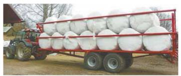
Trailer's retractable side rails eliminate the need for straps when hauling big bales. This 40-ft. model can carry up to 30, 4-ft. dia. round bales or up to 60 big squares.
