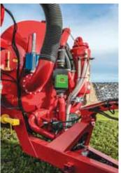
Sensor mounted on injector toolbar measures nutrient content in manure as it's applied.
