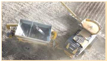
Grain is unloaded by the combine auger into hopper on front of cart, where a bubble-up auger moves it back. Power is provided by an engine on back of cart.
