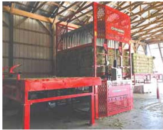
Chinook dryer can dry big square bales from 20 percent moisture down to 12 percent in just 10 min. It injects heat into bales using a 7,500 cfm fan.
