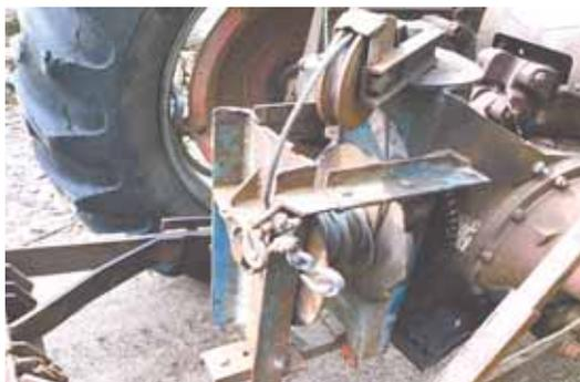
Winch spool assembly bolts to Farmall's drawbar and is chain-driven off tractor's pto.
