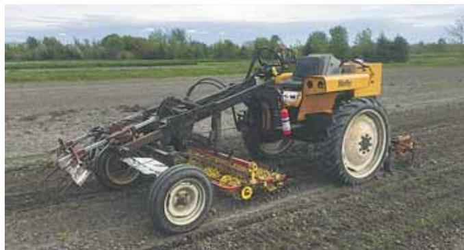
Reid Allaway replaced the Renault engine on his Hefty-G cultivating tractor with an 8-in. dia. DC motor and controller off old forklifts.
