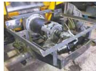
Tractor's 40-volt lithium battery pack (left) is made up of second-hand units purchased at an auction. Electric motor can deliver up to 20 hp. under maximum load.
