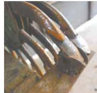
Jig is used to replace worn out spoke tips with Ho-Bit spoons, using a spoon holder that pivots into position for welding the Ho-Bits in place (left). Photo at right shows one spoon already welded on.
