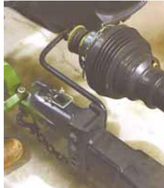
Rinke enclosed the wheel swivels and bearing spacers on his batwing mower with rubber pieces cut from shock absorbers, which keeps them clean (left). A swivel arm made of silo reinforcing rod mounts on mower hitch and holds the pto shaft when it's disconnected from tractor.
