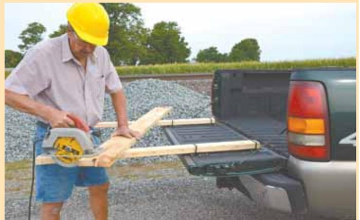
Tailgate Sawhorse uses a pair of 2 by 4 boards to extend pickup's tailgate by 3 ft. Kit includes 4 metal brackets and mounting hardware.
