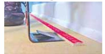
Zenith Trim Puller comes with a 15-degree center-mounted wedge that helps push out the trim.
