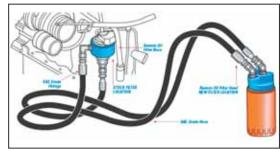
Kit moves the oil filter out into an open area for easier oil changes.
