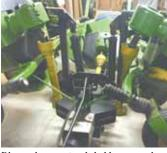
Diagonal support rods hold mower wings tight to mower's main frame.
