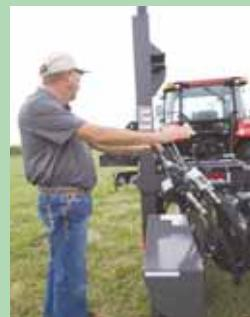
**Unit's** 750-lb. hammer can drive in posts up to 12 in. dia. and 12 ft. long.
