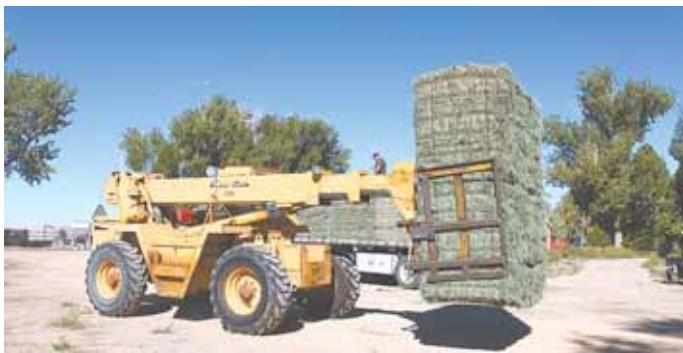
Cat loader-mounted bale fork uses a pair of hydraulic-operated squeeze arms attached to a steel backstop. It's designed for use with 21-bale bundles of small square bales.
