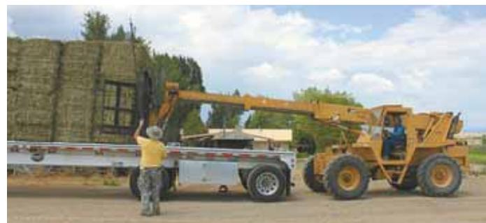
Bale fork quick-taches to Cat loader's extend-a-boom forklift.
