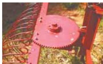
Big sprocket bolted on front of rake is used to adjust rake angle up to 45 degrees to either side.
