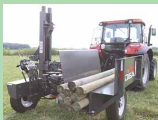
**Post pounder** sets on a trailer that can be pulled with a pickup or utility tractor, and includes a bin to hold posts.
