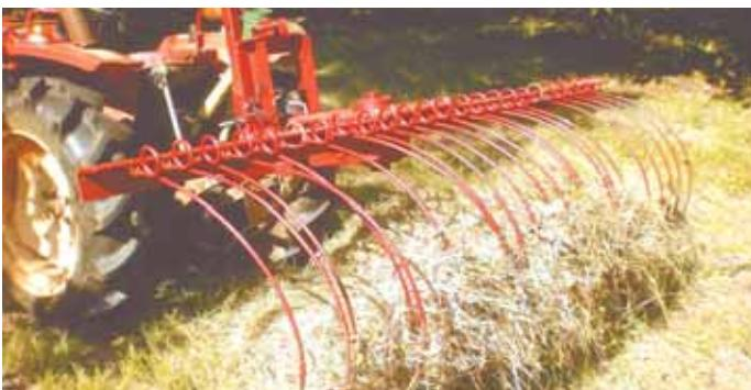
Glenn Fisher converted an old IH 8-ft. wide, horse-drawn rake to a 3-pt. mounted "yard rake". He uses it to rake leaves and grass, as well as pruned grape vines.
