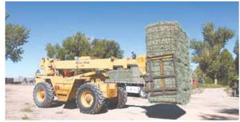
Cat loader-mounted bale fork uses a pair of hydraulic-operated squeeze arms attached to a steel backstop. It's designed for use with 21-bale bundles of small square bales.
