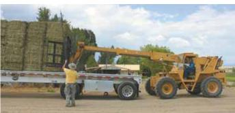
Bale fork quick-taches to Cat loader's extend-a-boom forklift.
