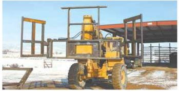
Sasser says the bale fork works great for stacking onto pickups, flatbeds and semi trailers.
