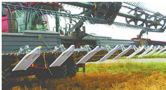
Bean shields bolt to spring-loaded crop lifters that attach to header.
