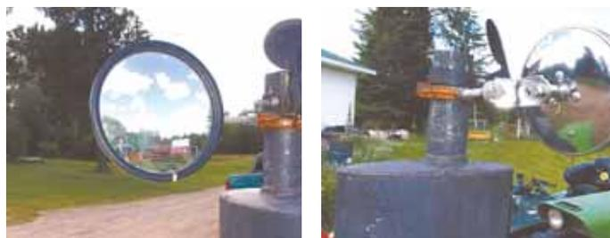
Muffler-mounted bracket supports mirror by means of a 1 1/2-in. pipe hanger and a 6 1/2-in. bolt.
