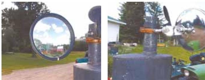
Muffer-mounted bracket supports mirror by means of a 1 1/2-in. pipe hanger and a 6 1/2-in. bolt.
