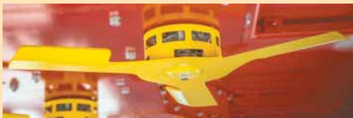
Bourgault's BTT Weed Clipper is designed to chop down weeds growing above the crop. It's fitted with hydraulic-driven rotary blades that work at high travel speeds.
