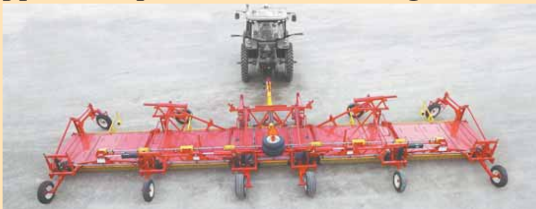
Bourgault's BTT Weed Clipper is designed to chop down weeds growing above the crop. It's fitted with hydraulic-driven rotary blades that work at high travel speeds.
