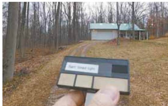
Andy Kozlowski uses a recycled garage door opener to turn on the lights outside his barn. A timer built into the opener shuts the lights off automatically.
