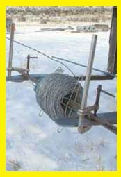
Here are a couple ideas we use for rolling and unrolling fence wire to maintain the 27 miles of fencing we have on our Central Idaho ranch. If you can get near the fence with a loader tractor, we put a set of forks on the front of the bucket and use two large adjustable clamps to hold a bar in place on top of the tines. We use a 6-sided
