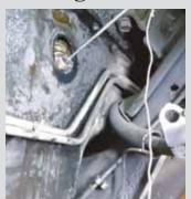
Heavy braided fishing line is tied to the end of a gun barrel cleaning brush, to keep the bulkhead from dropping into the oil pan.
