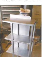
Chainsaws are stored on one side with oil and fuel cans on the other side. Chainsaw bars extend through gap at the back.
