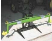
Front axle extensions for Deere "vegetable tractors" widen the front wheels to match the rear wheels.
