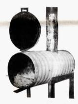
face area for radiating heat, making the stove more efficient. Because the culvert is 2 to 3 times as thick as the metal in a steel barrel, the stove is expected to last much longer than a common barrel stove.
