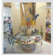
So I built a storage carousel that keeps my tools readily accessible, yet I can quickly move it out of the way if necessary. I keep the carousel on a nearby table.
