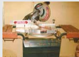
**Frank Brossart, Rugby, N. Dak.:** "I converted an old gas grill that didn't work any more into a portable table saw stand. I replaced the grill with a piece of 1/2-in. thick plywood and set the saw on top of it."
