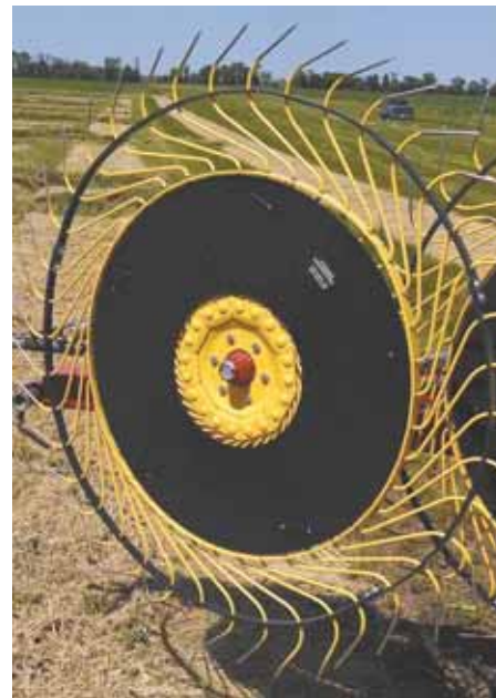
Silencer consists of 1-piece plastic bands that slip over rake wheel teeth and bolt together on the ends. Bands reduce damage to teeth in rough conditions.
