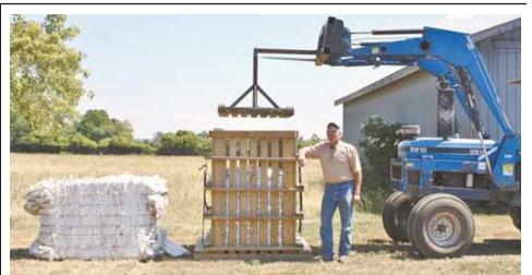
Lynn Leavitt with his "Pac-it" bale wrap compactor. Plunger attached to front-end loader compresses plastic as it's added to wooden box. Tied-off plastic bale is shown at left.
