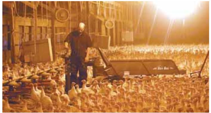
Machine’s rounded front allows gentle movement among turkeys. Operator makes use of a “leaning post” that doubles as a toolbox.
