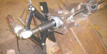
Brian Lough needed to enlarge the bore of the pin holes on his 12-in. used excavator bucket, so he built his own line-boring machine. He uses a scissor jack to align it and apply pressure.
