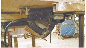
To keep the saw running continuously, he wrapped a metal bracket around the trigger and slipped a small wood wedge under it. To stop the saw, he just pulls out the wedge.
