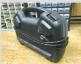
Ryan Van Der Bill, Sioux Falls, S. Dak.: "Instead of trying to stuff a tool's electric cord inside the tool case box, just wrap the cord neatly around the outside of the box. You might have to cut a small groove in the plastic where the box folds up in order to run the cord through."
