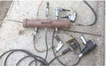
Mobile air splitter is made from a large heavy-gauge pipe with ends welded in place, and holes drilled in the sides to connect air lines.
