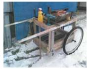
Tool cart rides on bicycle tires mounted to a frame built from broken pallets, with hockey sticks for handles.
