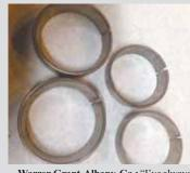
Warren Grant, Albany, Ga.: "I've always had trouble pushing new races back into place when a bearing goes bad. To solve the problem, I take a Dremel tool fitted with a small cut-off blade and cut through one side of the old race. It makes the race flexible enough that I can push a new race in and then remove the old one with little effort. Every time I change out a race, I save it so that I'll have various sizes on hand."
