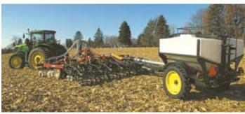
Verti-Seed Cart converts field cultivators, disks and other tillage toolbars into cover crop seeders that can till and seed in one pass.
