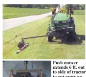
Push mower extends 6 ft. out to side of tractor to cut grass on ditch banks (above). Deck is suspended from a pair of short chains that allow mower to flex sideways.
