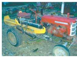
**Clifford Smith** mounted a 22ton wood splitter alongside his Farmall Cub. Once he's onsite, he rotates splitter to operate vertically.
