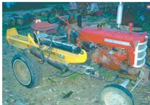
Clifford Smith mounted a 22-ton wood splitter alongside his Farmall Cub. Once he’s on-site, he rotates splitter to operate vertically.
