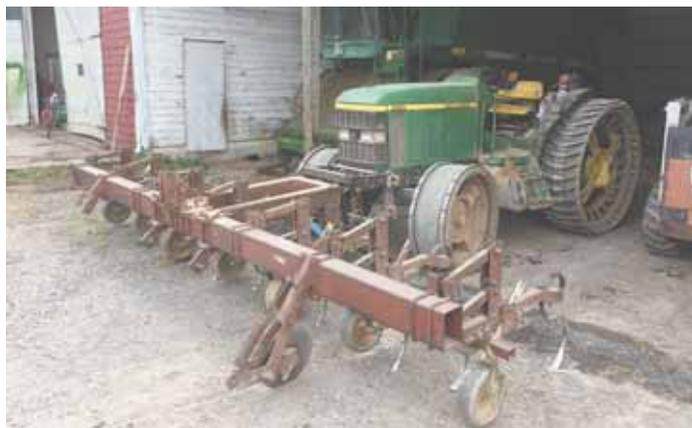
Last summer a Pennsylvania Mennonite farmer hooked up his cultivator to an Edwards front-mount 3-pt. hitch, designed specially for small tractors.
