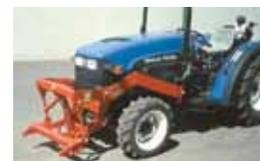
clutch housing to help support the load. A single hydraulic cylinder is used to raise and lower the hitch.
