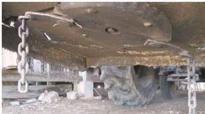
Taylor cut bush hog’s blades down to a 9-in. length, then welded lengths of heavy log chain onto blade ends. “I’m amazed at how well the chains chop up material,” he says.
