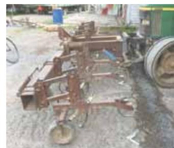
The 3-pt. hitch bolts on in place of tractor’s front weight bracket and can be set up for use with any Cat. I or II 3-pt. mounted implement.
