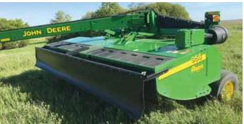
Rubber "curtain" bolts on in front of rotary/disc-style mowers, hay cutters and conditioners, protecting tractor and driver from flying rocks and debris.
