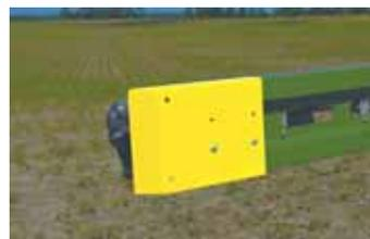
**Boomsaver guard protects boom ends, nozzles and hoses on Deere sprayers from damage caused by obstacles along edges of fields.**
