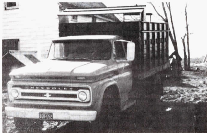
For hauling grain, air scoop provides about 8 in. of clearance to deflect wind.
