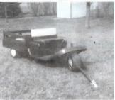
I made a handy utility pull-cart out of an old golf cart that no longer ran. I removed the body of the cart behind the seat and lengthened the frame by 24 in., moving the rear axle back. Then I fitted it with a wood cargo box and attached a wagon tongue to the single front wheel and fitted it with a ball hitch.
