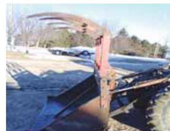
He relocated tractor's gas and hydraulic oil tanks to the back. Loader can be equipped with a home-built snow bucket, grapple fork, or 4-tine fork that can handle two 800-lb. big square bales.
