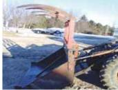
He relocated tractor's gas and hydraulic oil tanks to the back. Loader can be equipped with a home-built snow bucket, grapple fork, or 4-tine fork that can handle two 800-lb.
