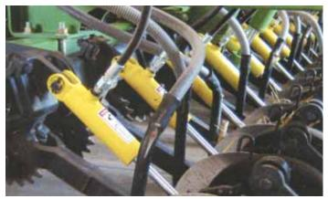
UniForce hydraulic down pressure system is designed for Deere drills. Single-action cylinders on each opener keep down pressure constant on uneven ground.
