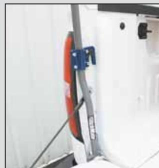
**Hitchmate Grab Handle** attaches to tailgate latch pin and hinge, providing a sturdy post with a hand grip above the bed sidewall. It can be used on either side of pickup
