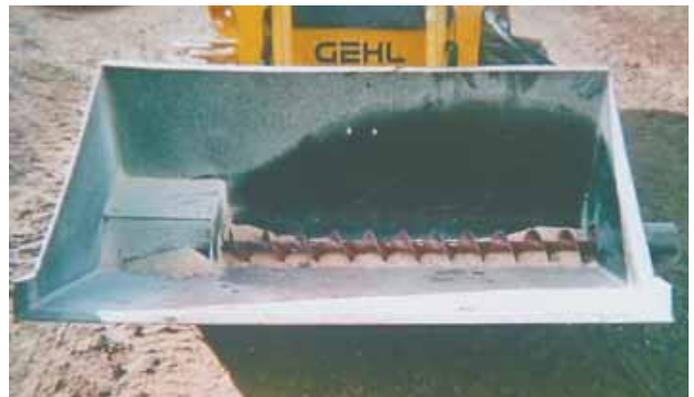
Home-built skid loader bucket is equipped with an auger and side chute that makes filling feed bunks an easy job.
