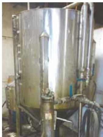
He had a local metal fabricator make this 400-gal. reactor equipped with pumps and heater.
