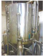
He had a local metal fabricator make this 400-gal. reactor equipped with pumps and heater.
