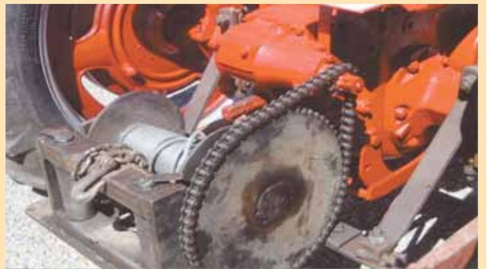
Winch spool assembly bolts to Farmall's drawbar and is chain-driven off tractor's belt pulley driveshaft.
