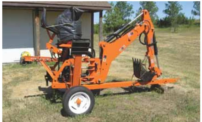
Ligtenberg converted the tongue, wheels and axle off a pull-type hay rake into a handy trailer, that makes his 3-pt. mini backhoe easier to hook up and store.
