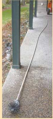
Flexible 20-ft. long CPVC pipe has a chimney brush attached to one end, allowing deVries to clean chimney from inside the house.
