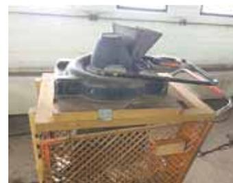
Roots are washed in a rotating drum, then sliced and spread on racks to dry (left). Feddema converted an electric lawn mower into a mill for grinding dandelion coffee.
