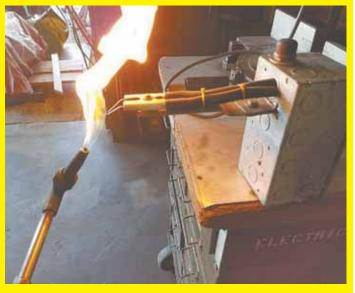
Torch strikers are a pain in the neck to use, especially as they get older and become less reliable, so I made my own low-cost ignitor from an old torpedo-style space heater. It operates on 110-volt electricity. I keep it on my welding table where it's always handy.
