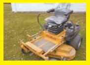
bit to make the bolts fit. I wired the seat to the mower battery to power the seat's air pump. A lever on front of the seat is used to raise it up or down. The lower the seat, the softer the ride.
