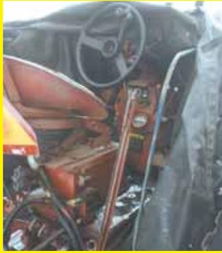
When my Comfort Cover tractor heater wore out, my son said, "Just use one of your fitted gravity wagon tarps." So I attached the 6 by 10-ft. tarp to the framework of the old Comfort Cover, and used tarp straps to hold it in place. It keeps the platform and seat snow and ice-free, and I stay warmer. Works great. **(Gary Swenson, Yankton, S. Dak.)**
