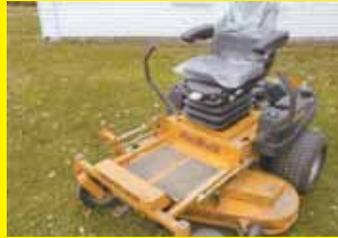
bit to make the bolts fit. I wired the seat to the mower battery to power the seat's air pump. A lever on front of the seat is used to raise it up or down. The lower the seat, the softer the ride.
