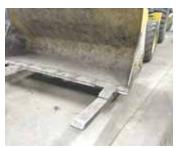
Harley Willmert made 2 bolt-on forks for his loader bucket in order to handle big logs. Forks go all the way under bucket and bolt onto its back side.
