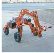
Robot uses a mechanical arm with chainsaw to cut tree flush with ground. A GPS unit helps it locate trees that a drone has previously geolocated on a field map.
