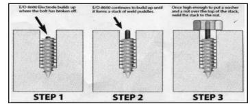
Kit contains a special welding electrode that builds up where bolt has broken off until it forms a stack of weld puddles. Once the stack is high enough, you weld a washer and a nut over the top of it.
