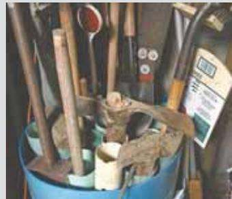
**Bob Payne, Coldwater, Miss.:** “To store long-handled tools, I cut the top off a plastic 55-gal. barrel and fill it with pieces of 4-in. dia. thin wall pvc pipe. The pipe holds the tools separate from each other. For D-handle tools, I just stick the D part down into the bucket between the pipes.”
